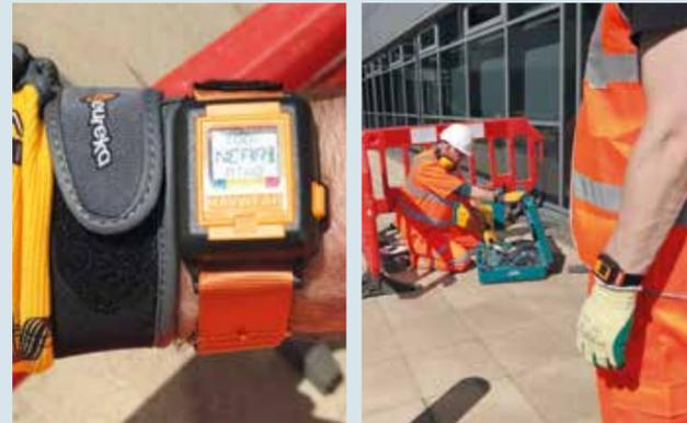
to detect other Reactec devices within a two-metre range. Should users become closer than two metres apart, both device users are warned with both vibration and audio alerts.
