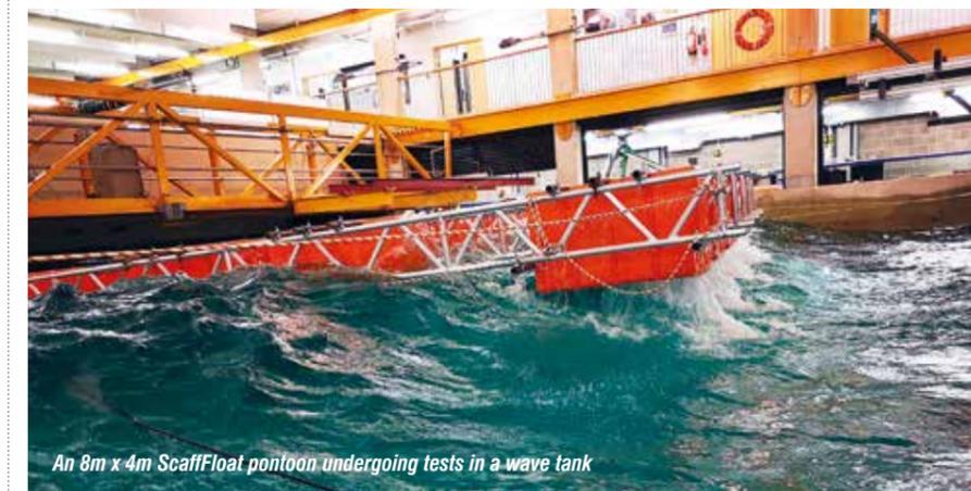
An 8m x 4m ScaffFloat pontoon undergoing tests in a wave tank
